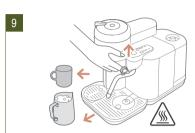
Once the coffee extraction and milk texturing are complete, remove the cup and milk jug from the machine.
