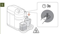
Press and hold the Steam Button for 3 seconds.
