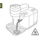
The machine will purge the steam wand once it returns to its downward position.
