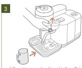
Lift up steam wand and insert in the milk jug. Position the milk jug, into the drip tray recess.
