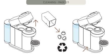
3 Unlock and open the machine and eject your used capsule\*. Empty and rinse the capsule container and the drip tray and put them back in place.
