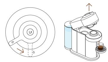
6 When the coffee stops brewing, open the machine head by turning the lever right towards the unlock position to automatically eject the capsule and enjoy your coffee.
