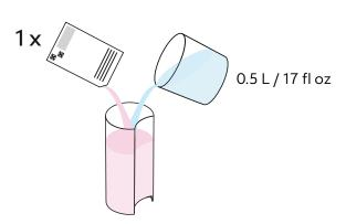
2 Fill the water tank with 0.5 L / 17 fl oz of water and add 1 unit of **Nespresso** descaling liquid.
