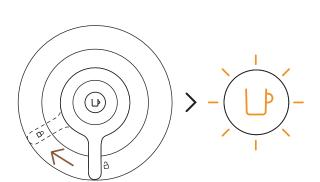
7 To enter the descaling mode, lock the machine by turning the lever left towards the lock position. The light should still be blinking orange quickly. This is an indication that you have entered descaling mode.
