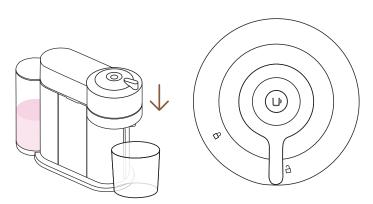
4 With the machine on, close the machine head and leave the lever in the unlock position.
