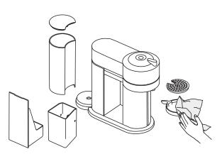
**11** Dry the machine with a clean and fresh towel. Let the machine dry for 10 minutes before using it.
