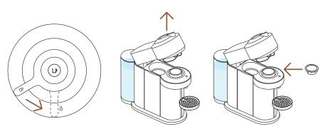
3 Unlock and open the machine head completely and insert a Vertuo capsule with the dome shape facing down.
