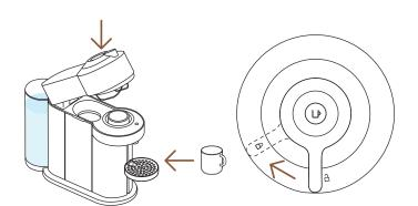
2 Close the machine head, turn the lever left towards the lock position and place a cup on the cup support.
