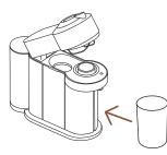
2 Place them back in position on the machine, remove the cup support and place an empty container (0.5 L / 17 fl oz) under the coffee outlet.
