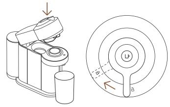
**3** With the machine plugged in, open and close the machine head and turn the lever towards the lock position.
