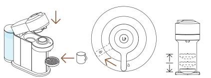
4 Close the machine head and lock by turning the lever left into the lock position and place a cup on the cup support. The cup support can be adjusted to accomodate your cup size.
