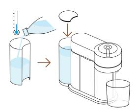
9 At the end of the descaling process, it is time to rinse the machine. Rinse the water tank and drip tray thoroughly. Fill the water tank with fresh drinking water and put it back in place. Empty the container and place it back under the coffee outlet.
