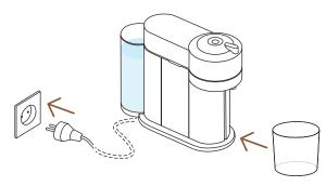
**3** Plug the power cord in, remove the cup support and place an empty container (of at least 1 L / 34 fl oz) under the coffee outlet.
