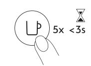
**2** Press the button 5 times within 3 seconds. The machine is now programmed with the factory settings.
