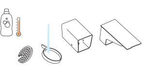
11 Wash the capsule container, the cup support and the drip tray with hot water and mild odourless detergent.
