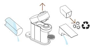
1 Empty the water tank, open the machine head, and let the used capsule be ejected. Empty the capsule container and the drip tray. Don't forget to recycle your **Nespresso** capsules.\*
