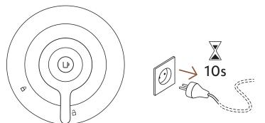
1 With the machine closed and the lever in **unlocked** position, unplug the machine for at least 10 seconds.
