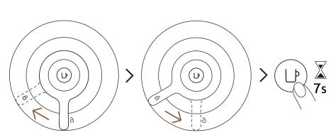
6 Lock the machine head by turning the lever left until the lock symbol and then unlock the lever by turning right to the unlock position. Press and hold the button again for approximately 7 seconds or until the light turns off. The button will start blinking orange rapidly.
